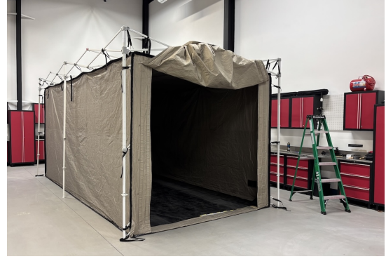
Figure 2: We drove the vehicles into this Faraday tent to block external cellular signals.
